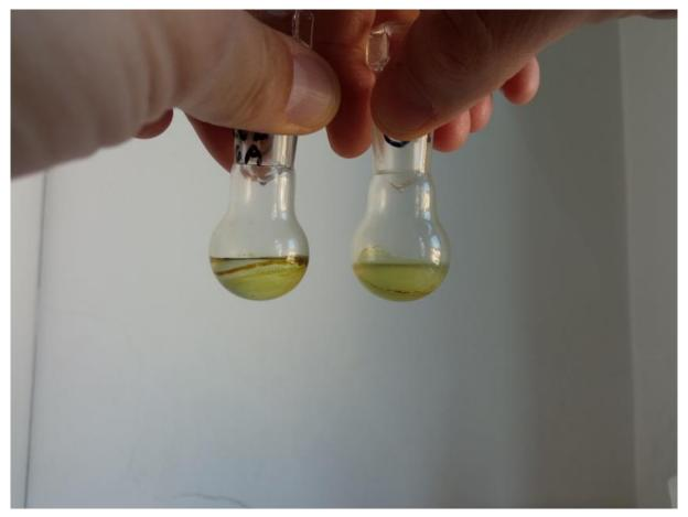
Figure 2: Comparison in water solubility between unmodified (left) and modified (right) hemp resin. Mitja Križman and Jure Zekič. 2022.
