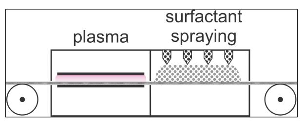
Figure 2: Proposed treatment process for producing antiviral textiles. Gregor Primc. 2022.
