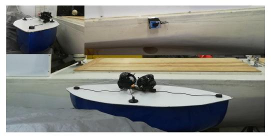
Figure 4: Mobile Elecromagnetic Mooring System (MEMS) – laboratory model in scale 1;30. P.Kolakowski. 2022.
