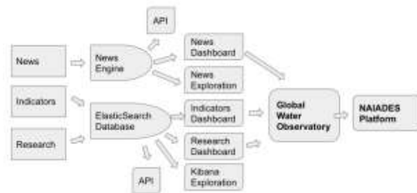
Figure 4: System architecture of the NIAIDES Water Observatory showcasing the relation between used technologies and NOW views
