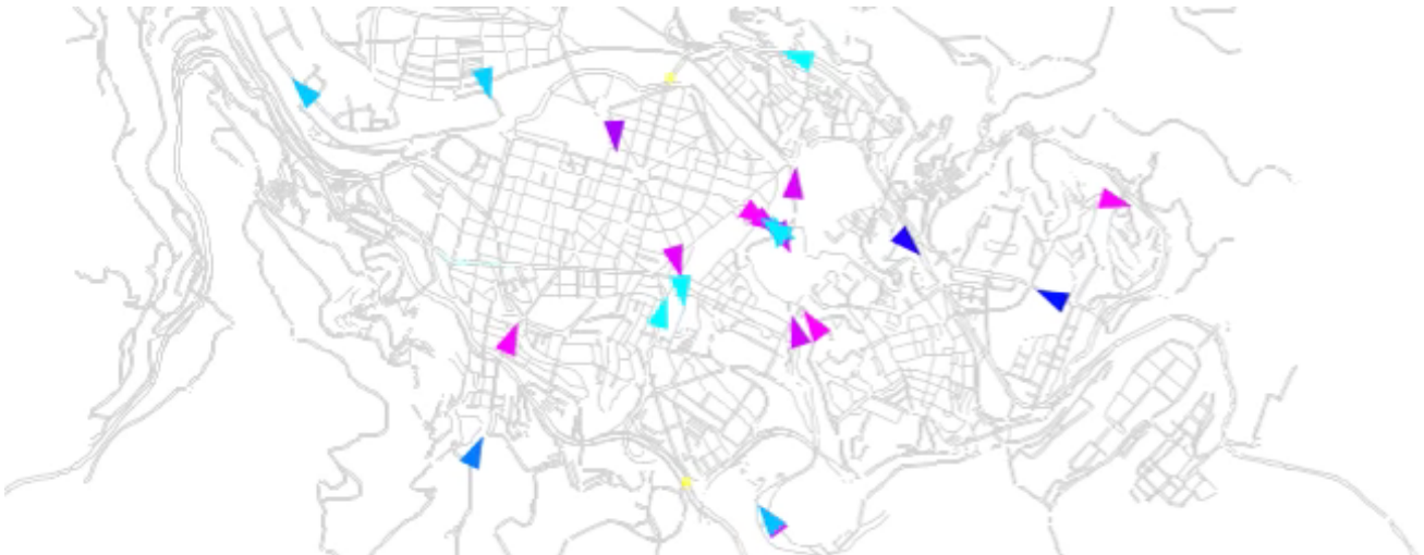
Figure 1: Part of a traffic simulation of Bilbao, made with MATSim. Triangles represent a sampled subset of the vehicles in the network, where cyan-colored vehicles are moving at high speed and pink-colored vehicles are stationary - either waiting at traffic lights or stuck in traffic.
