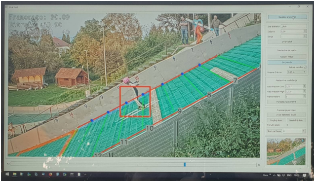
Figure 6: Trained operator determines the distance by using the calibrated measuring grid in 5-8 s.
