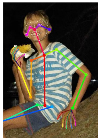
Figure 1. An example of the image processed by OpenPose. The Fingers, arms and facial characteristics are extracted and returned as points.
