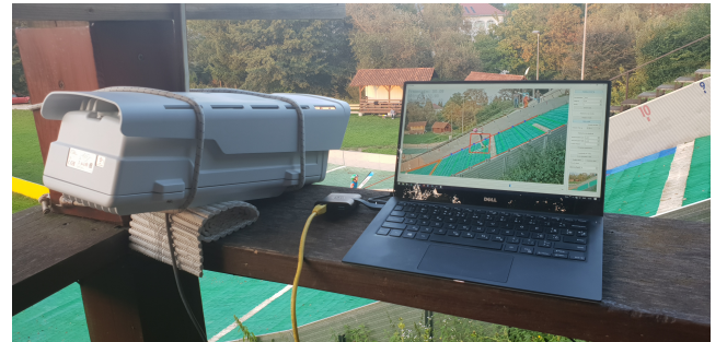
Figure 5: An online video distance measuring system consisting of a network camera (left) and a laptop computer.
