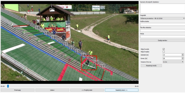
Figure 1: Offline video distance measuring system. A calibrated measuring grid is overlaid over video stream. Eight distance-measuring umpires can be seen standing along the landing slope.
