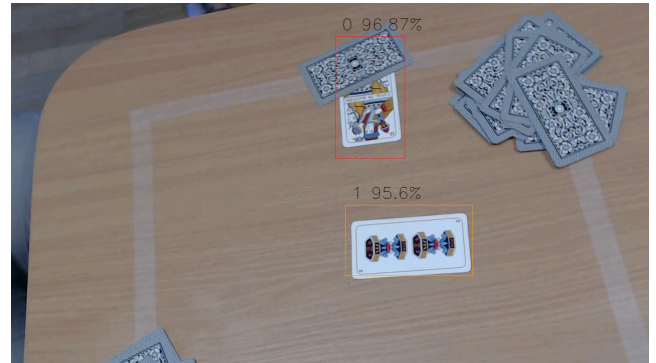
Figure 3: Detecting cards with YOLO is fast and reliable if objects do not overlap.
