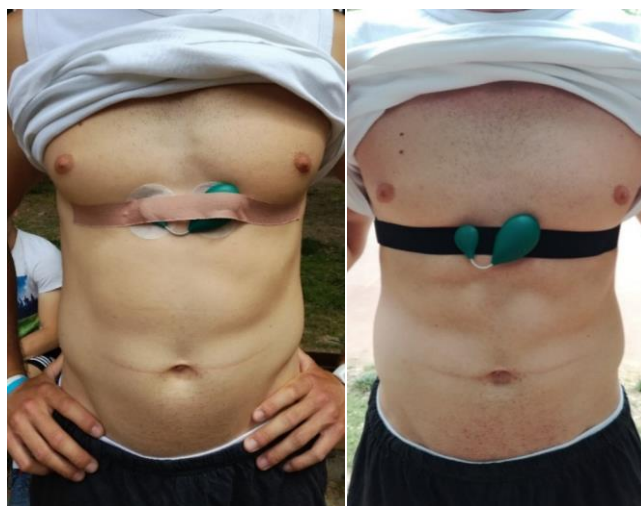
Figure 1. Sensor position and type of sensor fixation in the first test (left-hand) and in the second test (right-hand).
