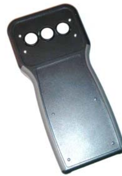
Figure 1: A mobile portable sensor pack developed for the CITI-SENSE project
