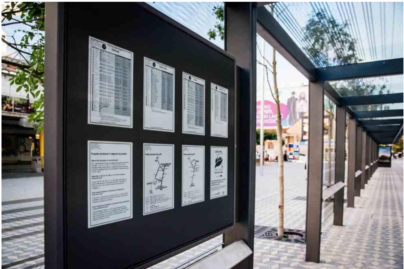
Image 1. Digitizing existing city services: electronic paper displays with passenger information at Ljubljana's bus stops.
