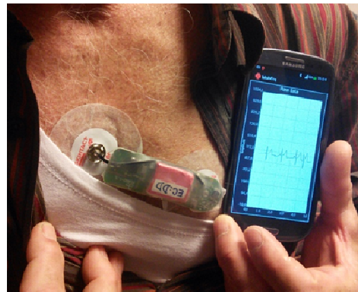
Figure 2. Prototype personal equipment of PCARD system: small body sensor and Smartphone.
