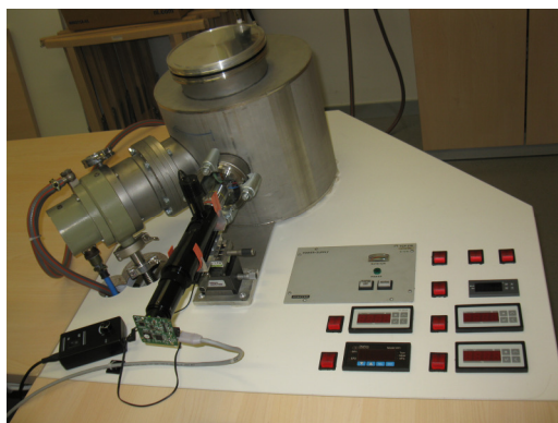
Figure 6: Vacuum chamber with an optical microscope
