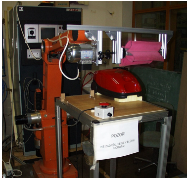
Figure 3: The cleaning materials evaluation setup.
