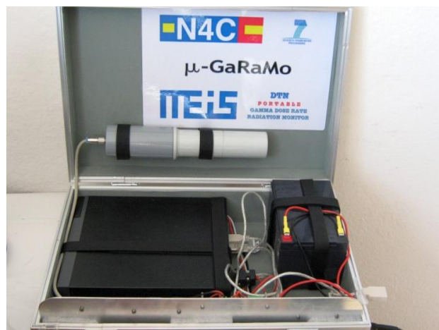
Figure 4: μ-GaRaMo DTN node for gamma dose rate radioactivity measurements
