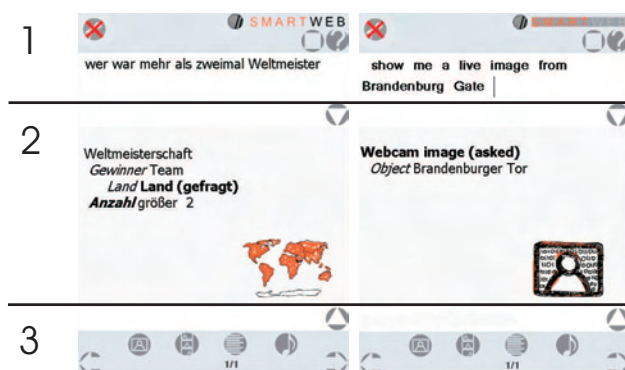
Figure 1: In (1) we display the output of the automatic speech recogniser, (2) shows the corresponding multimodal semantic paraphrase. The query paraphrase can also be listened to by on ear audio output. While audio repetition plays, barge-in is possible which leads to correction modes for single words or the complete query.
