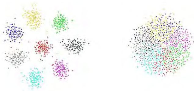
Figure 5: Pseudo-random graph with intra-cluster edge probability 0.16 and inter-cluster edge probability 0.01; left LinLog right FR
