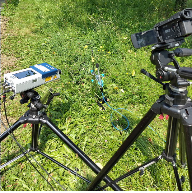
Figure 1: Data acquisition setup for recording vibration signals, audio, and visual recordings from flowers.
