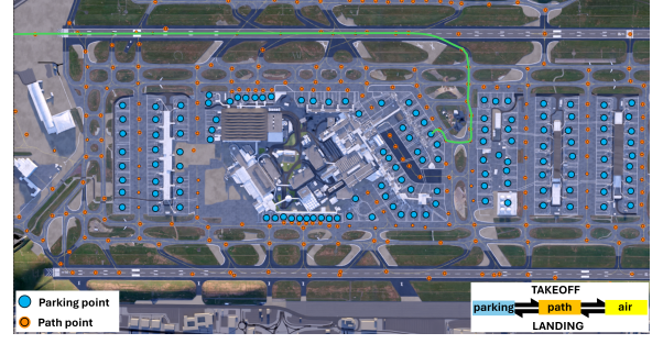
Figure 3: Top-view of the scene showing specifically positioned path points (orange) and parking points (blue). These points are used to establish randomized directional connections between neighboring nodes, to create realistic airplane movements. A sample generated trajectory is shown in green.
