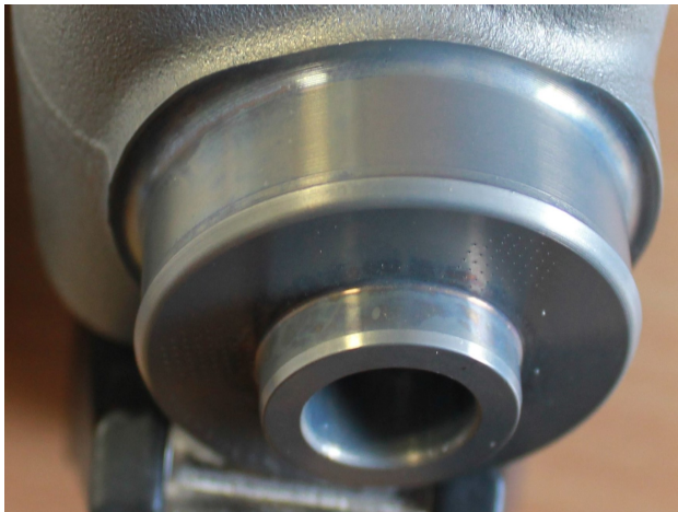
Figure 1: The object whose cylindrical polished surface we must examine for scratches
