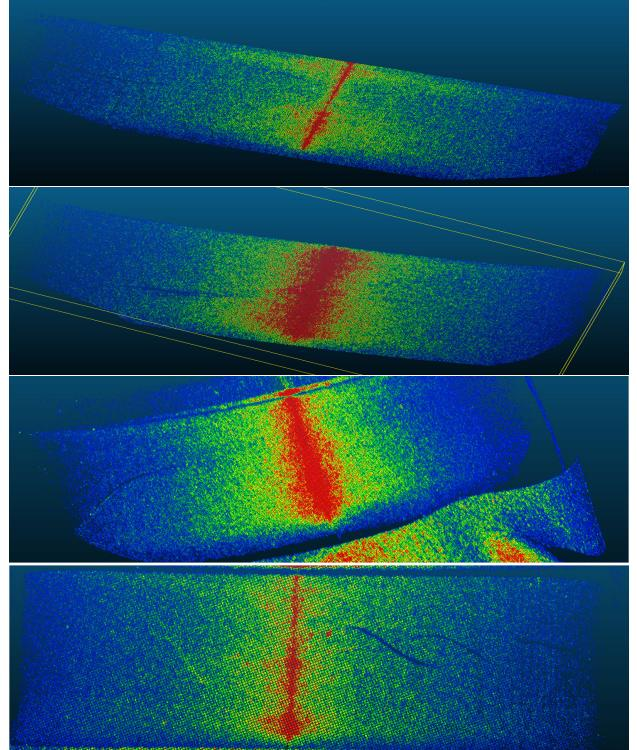
**Figure 3:** A visualization of several point clouds which show real-life objects with a visible scratch on their metallic surface.
