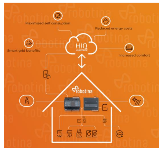
Figure 2: HEMS system operation and functionalities scheme.
