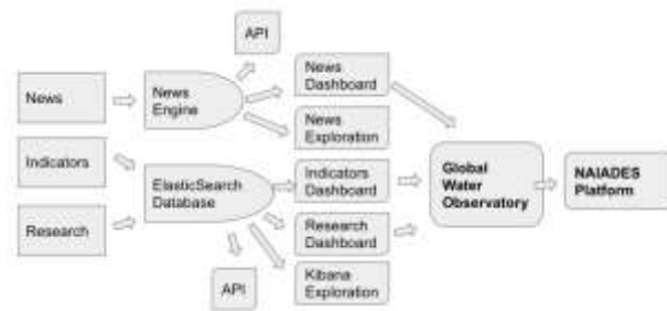
Figure 4: System architecture of the NAIADES Water Observatory showcasing the relation between used technologies and NOW views
