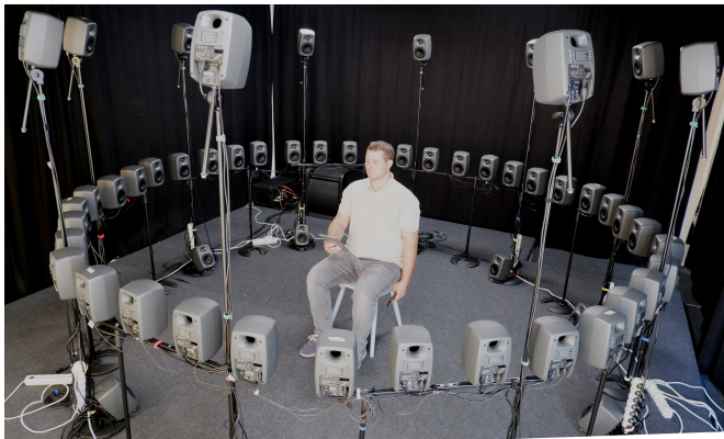
Figure 4: Photo of a listener in the Ambisonics loudspeakers ring at the InnoRenew CoE’s Acoustic lab. The control over the system and perceptual response is based on a tablet PC as an interface.
