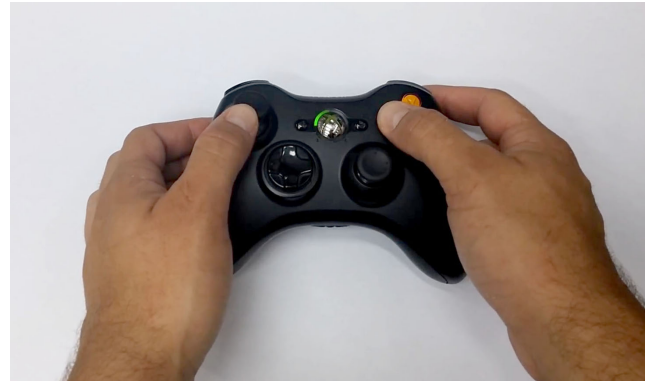
Figure 4: A consumer grade joystick interface that we used to perform precise motions of the robot in Cartesian space.
