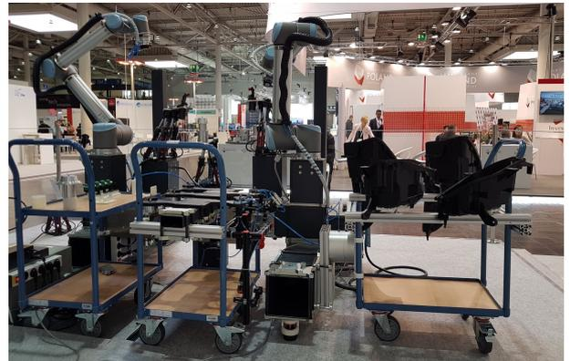
Figure 1: The proposed reconfigurable workcell prototype shown at Hanover fair 2017.
