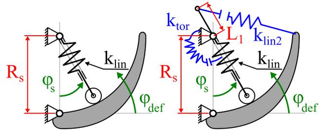
**Figure 4: The main device parameters (left) with the two proposed modifications (right).**
