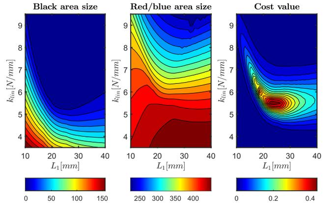
**Figure 8: Black, red-blue area sizes and the corresponding cost value for different  $k_{lin}$  and  $L_1$  parameter combinations.**
