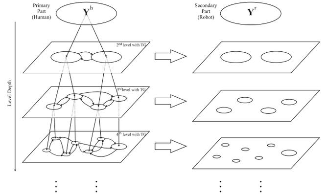
Figure 1: A simple representation of a dual database. The primary part, used for construction and motion recognition, can be seen on the left. The secondary part, seen on the right, stores corresponding robot movements.
