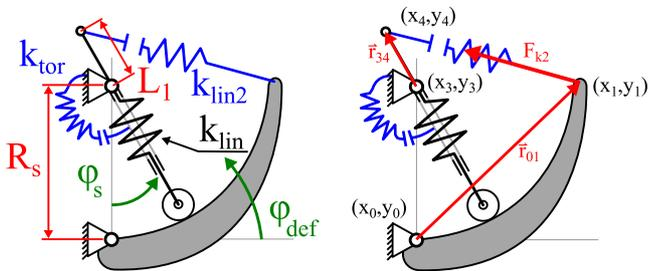
**Figure 6: A scheme of the proposed mechanism with the force and distance vectors.**
