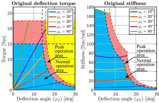
**Figure 2: Normal torque/deflection workspace and the corresponding stiffness graph.**
