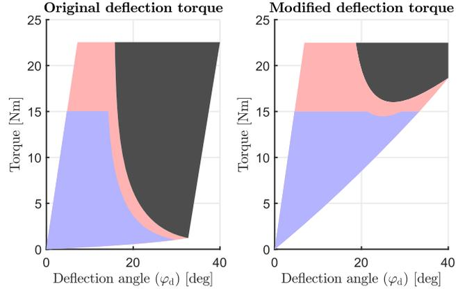
**Figure 7: Workspace comparison between the normal and modified mechanism version, where red-blue area is desired and black undesired.**
