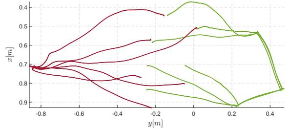
Figure 3: Set of demonstrated cooperative trajectories seen in two dimensions Robot trajectories, denoted in red, were converted to task space for presentation purposes. Human trajectories are denoted in green.
