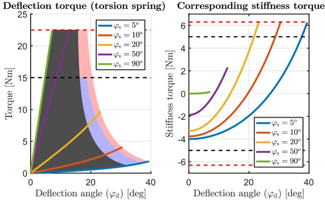
**Figure 5: Normal deflection torque (black area) and the new workspace with torsion spring (red-blue area). The corresponding stiffness torque is on the right graph.**
