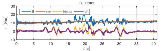
**Figure 3: The feed-forward torque on the first joint of the right robot, and separate components when using the complete controller, given by (15). See the bottom plot of Fig. 2 for the perturbation.**
