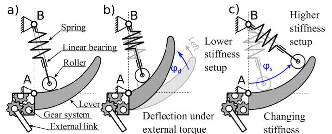
Figure 1: The actuator working principle: a) equilibrium position, b) deflection under external load, and c) varying stiffness.
