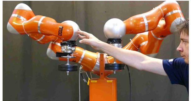
Figure 1: Bimanual robot performing a task while being perturbed by a human.
