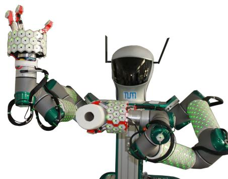
Figure 1: The robot TOMM [5] with two arms and two grippers covered with skin; the robot holds a paper towel in its left gripper which it uses to push the right arm; the right arm is controlled by our novel event-driven tactile reaction controller; it tries to avoid contacts and moves to the right.
