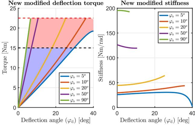
**Figure 9: The torque/deflection workspace for the new mechanism with the corresponding stiffness.**
