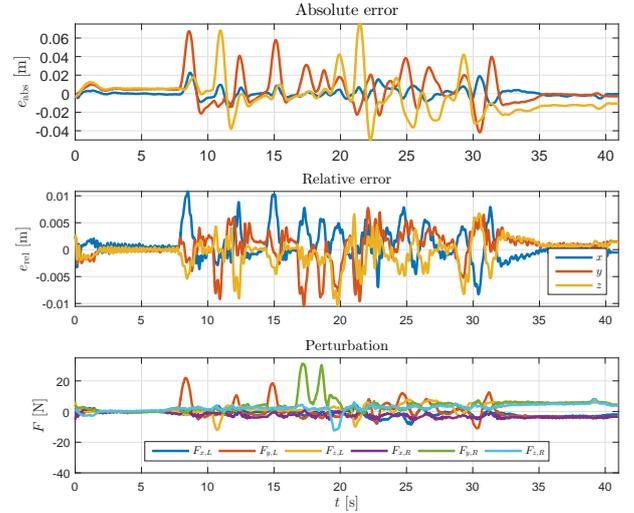
**Figure 2: Absolute error (top), relative error (middle) and end-effector perturbation (calculated from measured joint torques) when using the complete controller, given by (15).**
