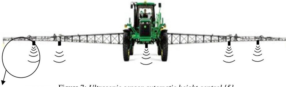
Figure 7: Ultrasonic sensor automatic height control [5].
