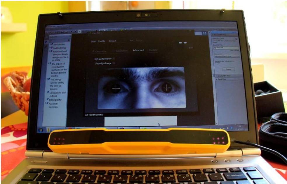
Figure 2: SMI's RED-m eye tracker and the application used to calibrate it.
